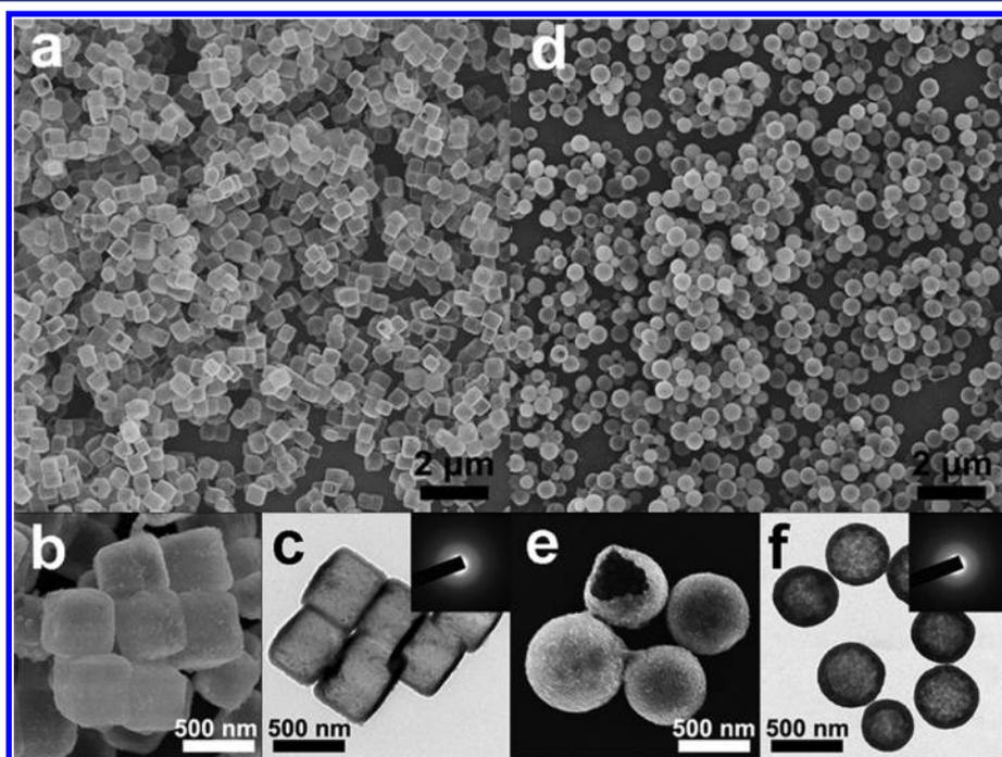
**Figure 8.** SEM and TEM images of  $\text{Ni}(\text{OH})_2$  nanocages with (a–c) cubic and (d–f) spherical structures. The insets in parts c and f are SAED patterns, indicating the amorphous feature of the samples.
