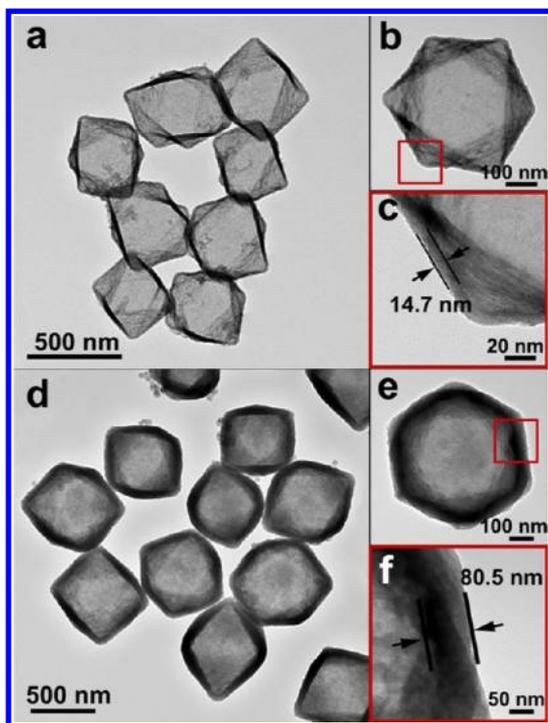
**Figure 7.** TEM images of the  $\text{Ni}(\text{OH})_2$  nanocages with shell thickness around (a–c) 15 nm and (d–f) 80 nm. Parts c and f are the magnified images of the typical shell structure from the marked areas of the nanocages in parts b and e, respectively.
