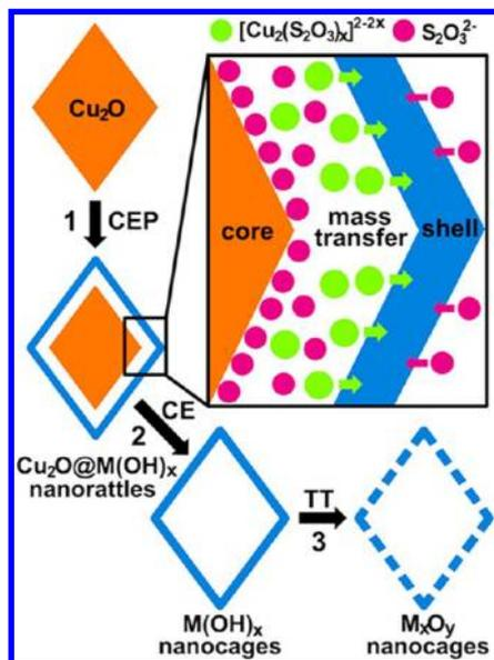
**Figure 1.** Schematic illustration of the fabrication of  $\text{M}(\text{OH})_x$  ( $\text{M} = \text{Mn, Fe, Co, Ni, Zn}$ ) nanocages by synchronous coordinating etching of  $\text{Cu}_2\text{O}$  nanocrystals and the fabrication of  $\text{M}_x\text{O}_y$  by thermal treating of relevant  $\text{M}(\text{OH})_x$ . Abbreviations used: CEP, coordinating etching and precipitating; CE, coordinating etching; TT, thermal treatment.
