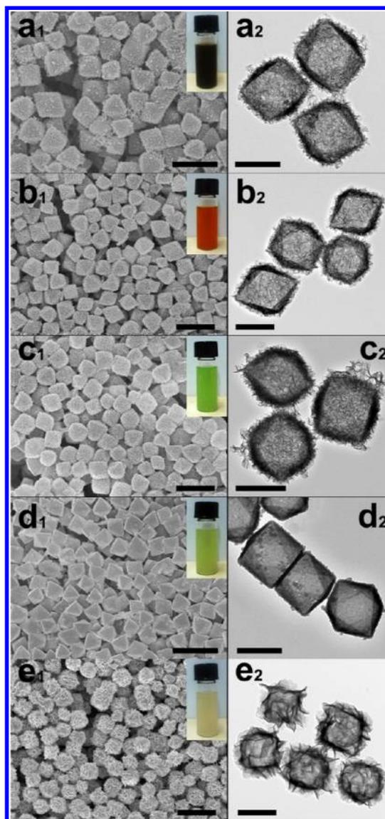
**Figure 3.** Overview SEM images and TEM images of the (a) manganese, (b) iron, (c) cobalt, (d) nickel, and (e) zinc hydroxide nanocages. Insets of  $x_1$  ( $x = a-e$ ) are digital photos and show the colors of the sample solutions. The scale bars in parts  $x_1$  and  $x_2$  are 1  $\mu\text{m}$  and 500 nm, respectively.
