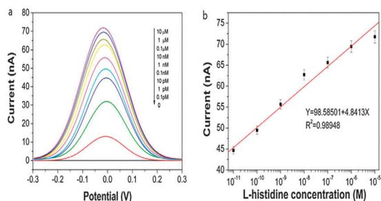
**Fig. 4** (a) Typical SWVs of sensing system to different L-histidine concentrations from 0.1 pM to 10  $\mu$ M. (b) Linear relationship between the peak currents and L-histidine concentration.
