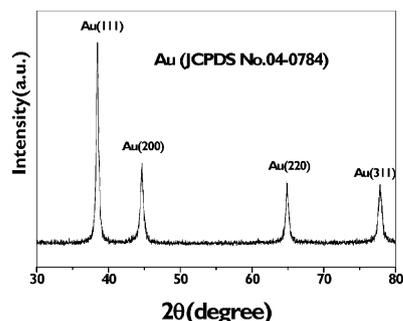
**Fig. 1** X-Ray diffraction pattern of GNPs–GNSs nanocomposite.
